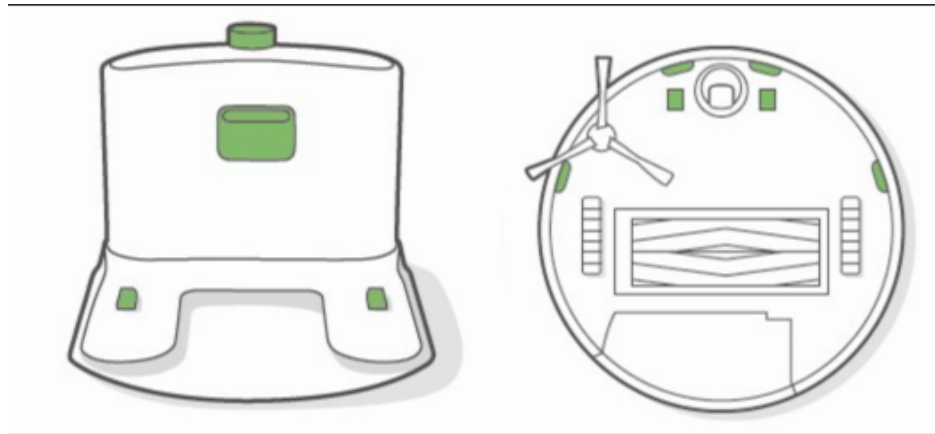
Figure 17: (Left) Docking Station. (Right) Roomba Contact Points
